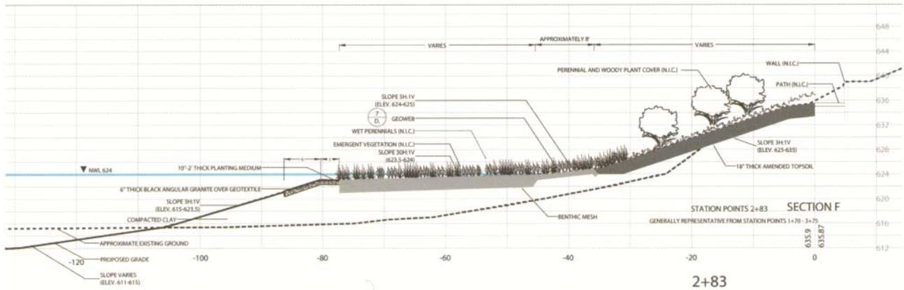
**Figure 1.** Cross section of shoreline. With the dual goal of repairing and beautifying the lake system, the designer developed a range of shoreline treatments: geotextiles for soil separation, geocellular reinforcement.
