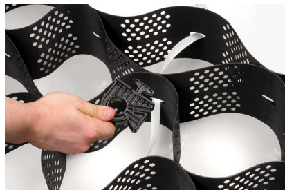
Figure 2. Inserting the ATRA® Tendon Clip through the GEOWEB Cell Wall I-Slot.
